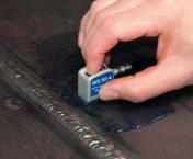
The new angle probes for non-destructive material testing of the angle probe series SONOSCAN check metals for cracks and inclusions. They are mainly used for weld inspection. The ultrasonic probes detect critical defects i.e. discontinuities and quality deficiencies of welds. The SONOSCAN probes are effective ultrasonic converters, which were adapted to the common mobile ultrasonic testing equipment.
