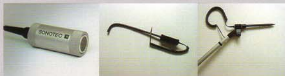
Air sound probe / Flexible probe / Telescope with air sound probe (range 3 m)
