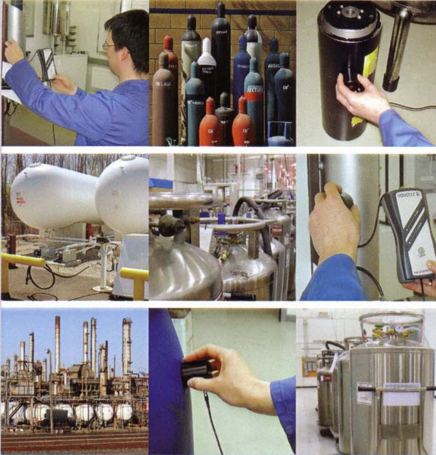
Fig. 1-3 level control at vessels, bottles and pipes
